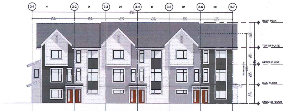
1 SOUTH ELEVATION - BUILDING 3 & 16 1:100
